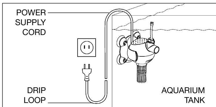
The "drip-loop" is that part of the cord below the level of the receptacle, or the connector if an extension cord is used, to
