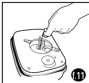
**Warning:** These motor units incorporate a ceramic impeller shaft. This shaft is permanently attached to its plastic holder for safe handling. The shaft is brittle to lateral pressure. Take extreme care when handling. Do not try to bend the shaft.
